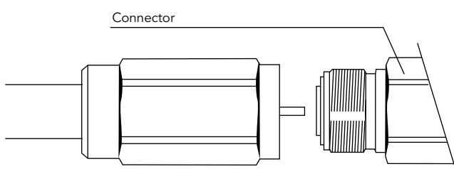
Pull the connector body over the cable's inner conductor and screw the nut tightly onto the connector body.
