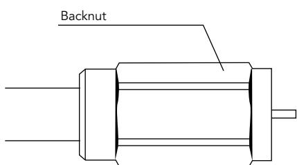
Pull the backnut over the cable as far as possible.
