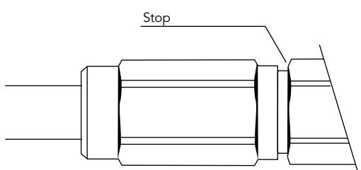
Please use two open-end wrenches. The nut is turned onto the connector body until it stops (metal against metal). Always hold the connector body while screwing the nut! Please find further information concerning wrenches within our tools catalogue
