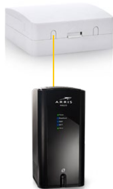
As demarcation point for third-party FO gateway
